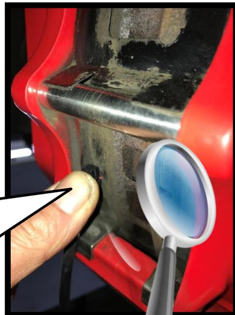
**🇬🇧** The sensor needs to be Manually installed and pressed by hand into the hole until it is secure
