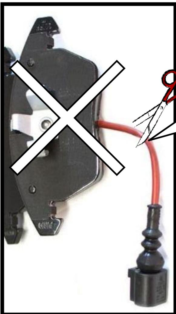
**🇬🇧** The original sensor connector needs to be cut from original brake pad
